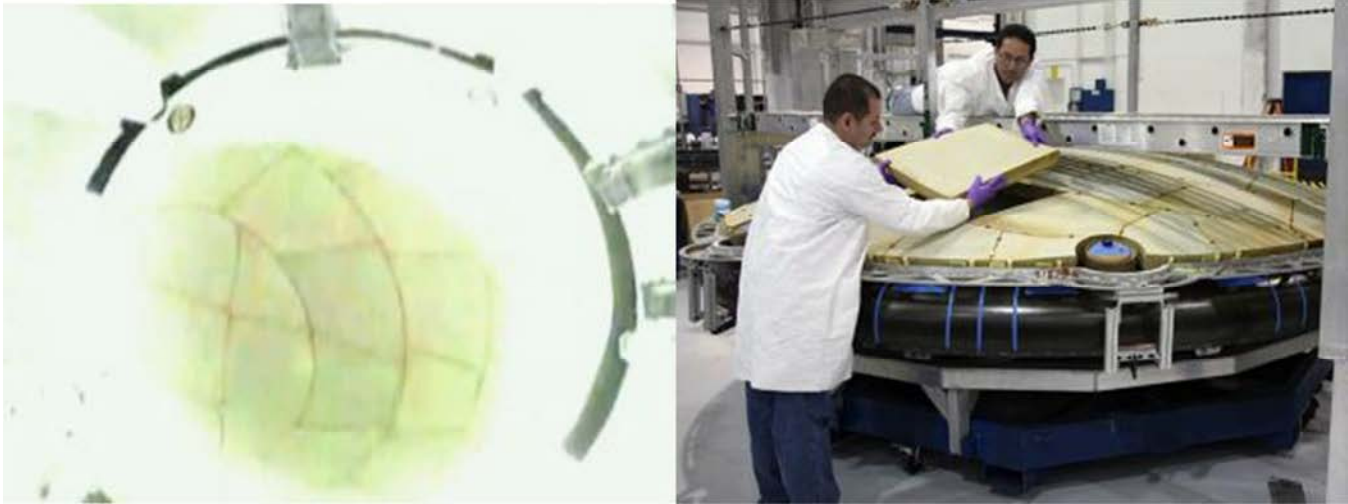
LEFT: Dragon's PICA-X heat shield (shown in flight) protected the spacecraft during reentry from temperatures reaching more than 3,000 degrees F. RIGHT: SpaceX engineers working on PICA-X heat shield, a SpaceX variant of NASA's original PICA formula.
