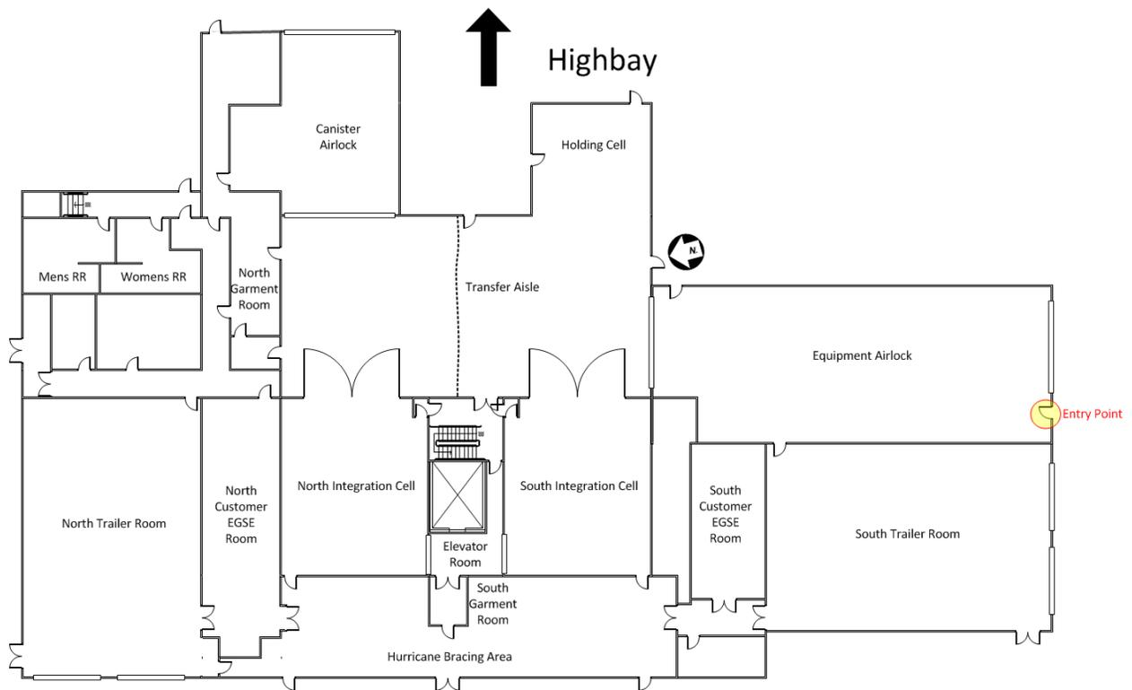
Figure 10-5: CCSFS PPF West Bay Floor Plan
