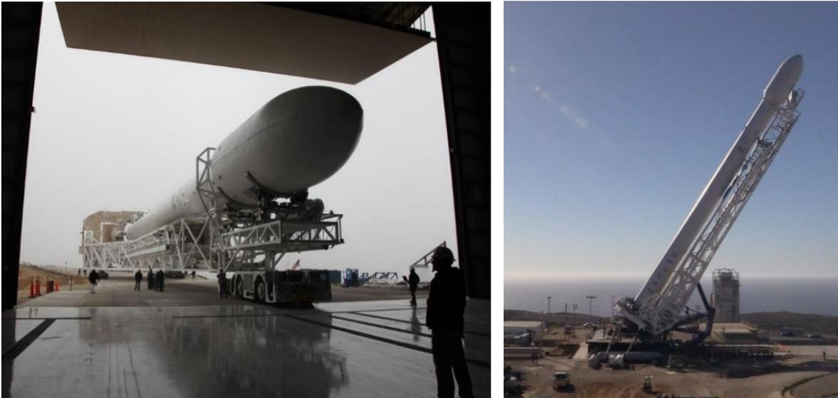
**Figure 10-10: Launch Vehicle Rollout and Erection**
