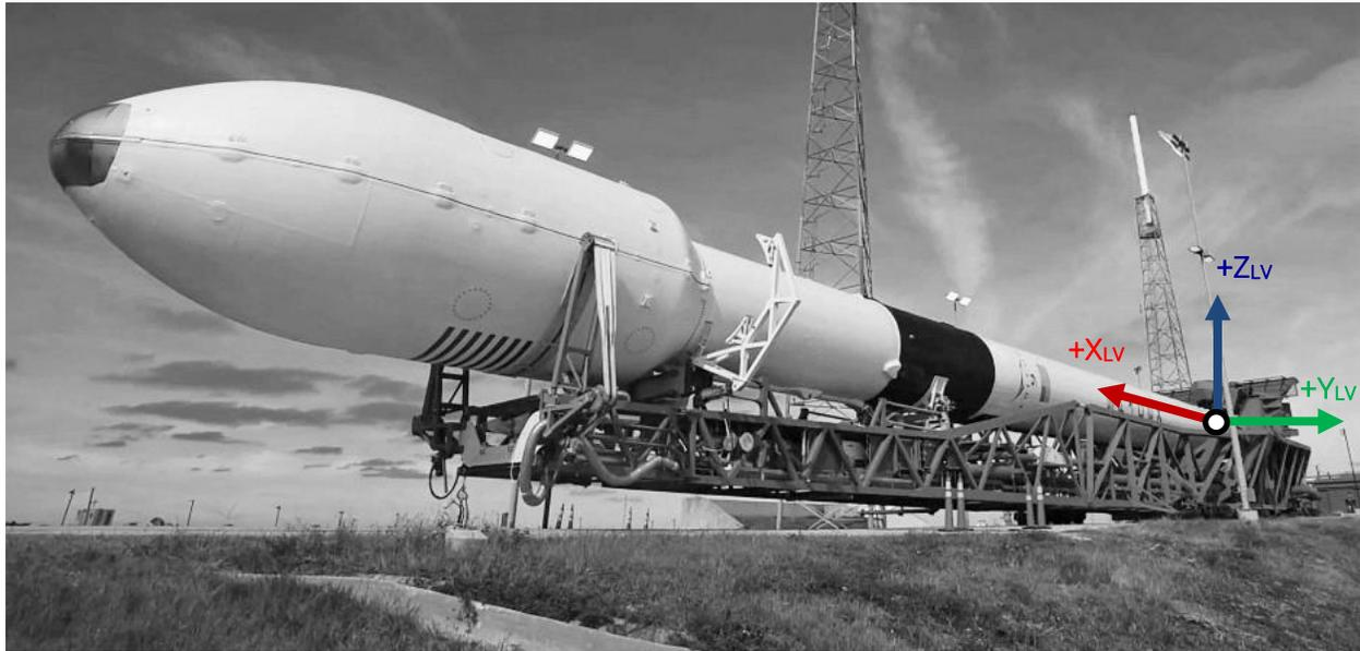
Figure 4-1: Launch Vehicle Coordinate Frame
