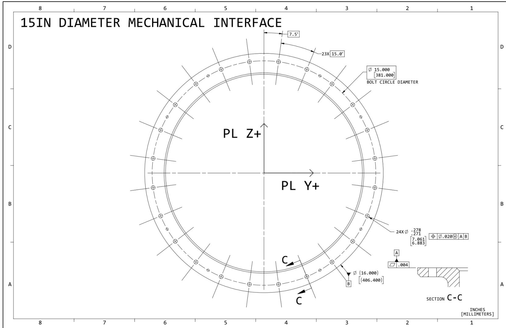
Figure C-1: 15" Diameter Mechanical Interface for Constellation Payloads
