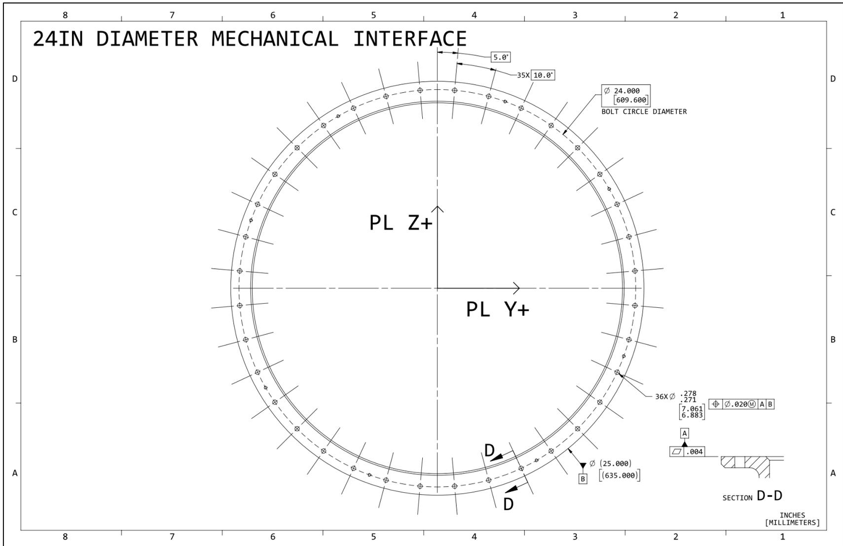
Figure C-2: 24" Diameter Mechanical Interface for Constellation Payloads
