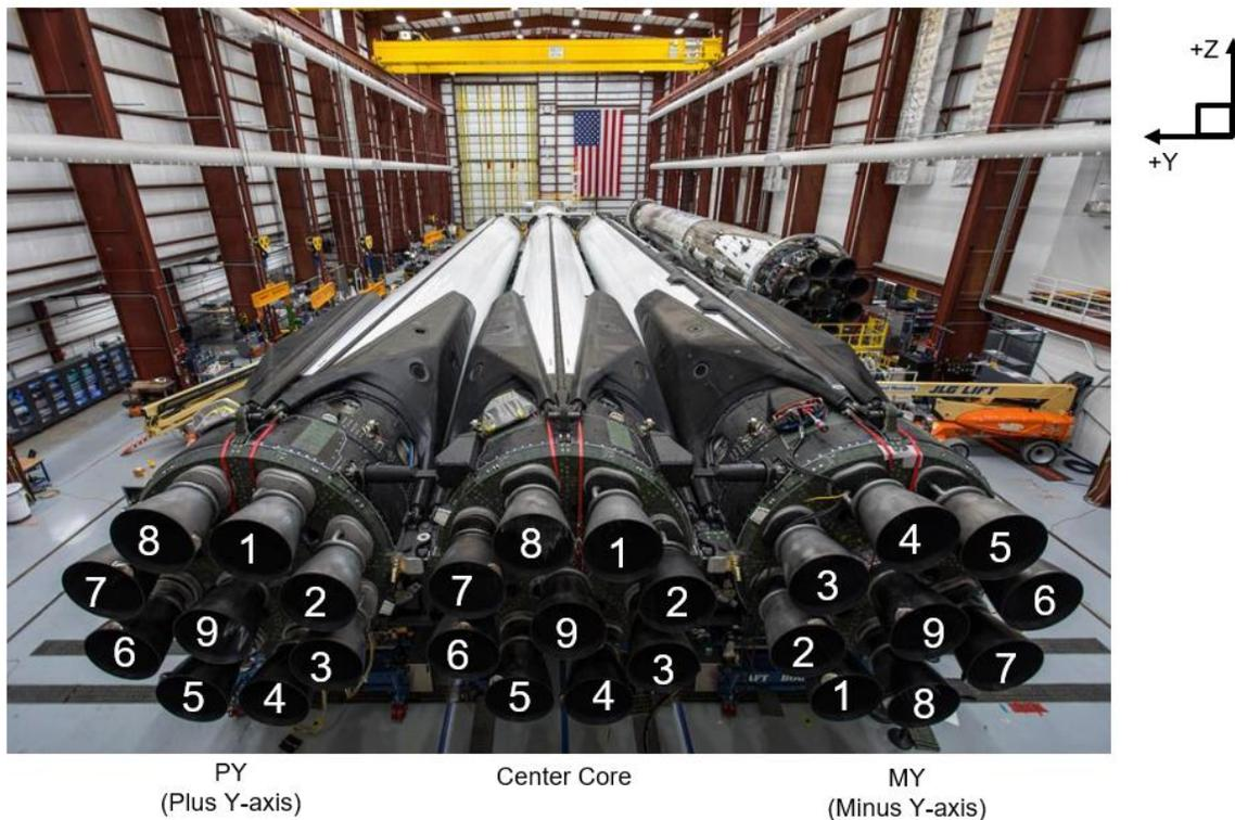
**Figure 2-3: Falcon Heavy First Stage Engine Layout**
