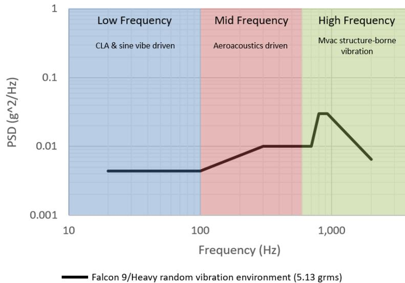
**Figure 5-7: Falcon 9/Falcon Heavy Random Vibration MPE**
