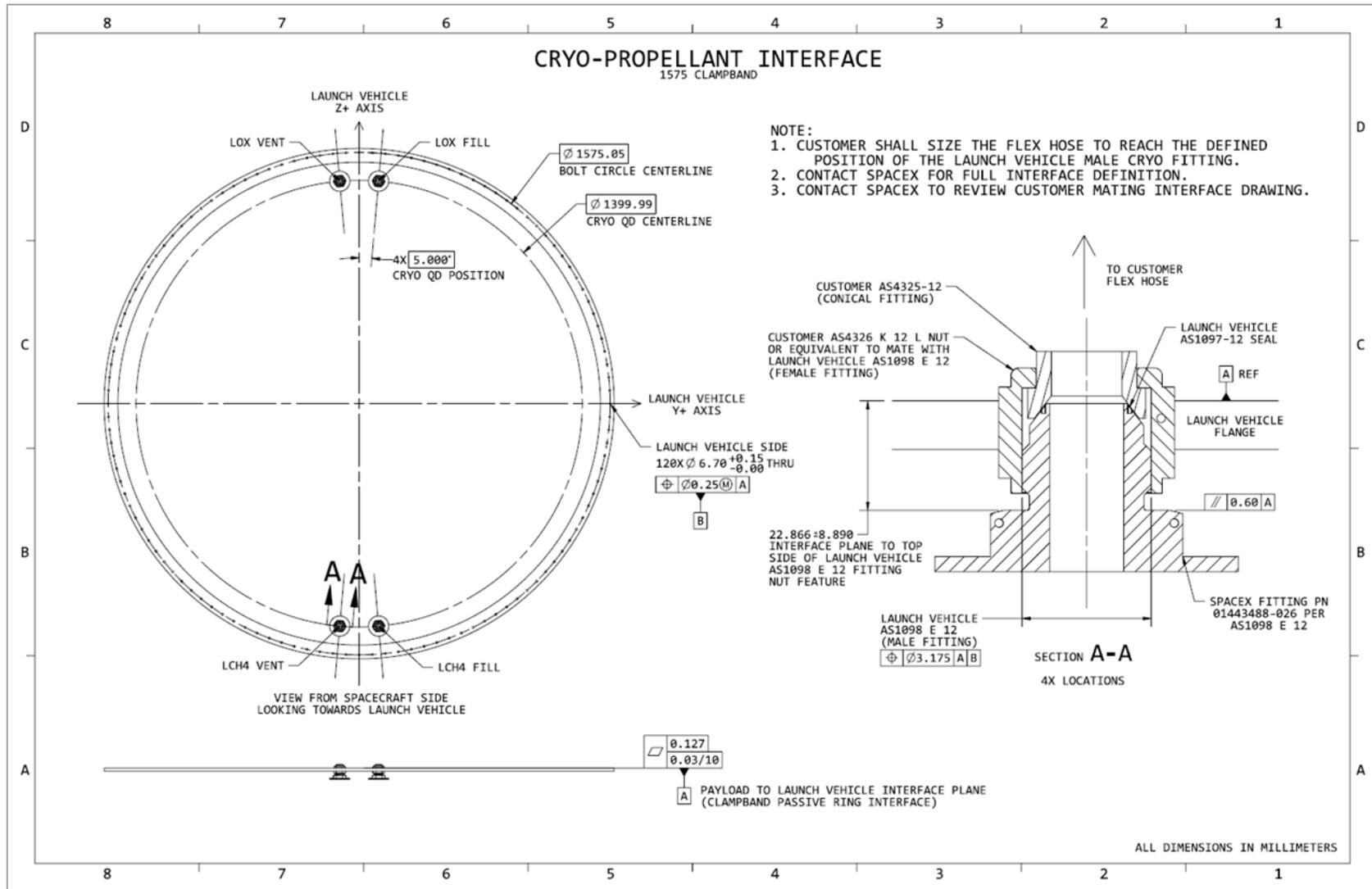
Figure D-1: Cryo-Propellant Mechanical Interface (1,575 mm Clampband)
