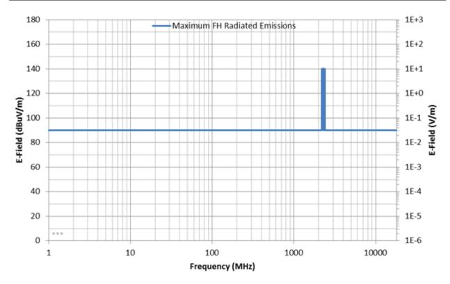
Figure 4-14: Falcon Heavy worst-case radiated environment
