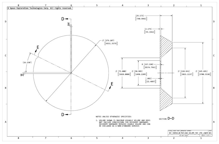
Figure 12-6: Payload lower volume, with 1,575-mm PAF (1 of 2)
