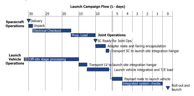
Figure 8-1: Illustrative Falcon launch vehicle processing, integration and launch operations schedule
