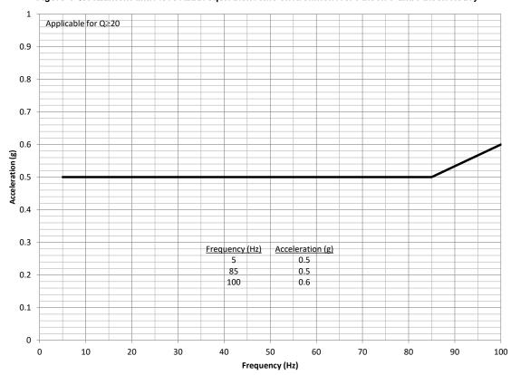
Figure 4-4: Maximum limit level lateral equivalent sine environment for Falcon 9 and Falcon Heavy
