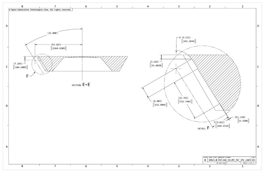
Figure 12-7: Payload lower volume, with 1,575-mm PAF (2 of 2)
