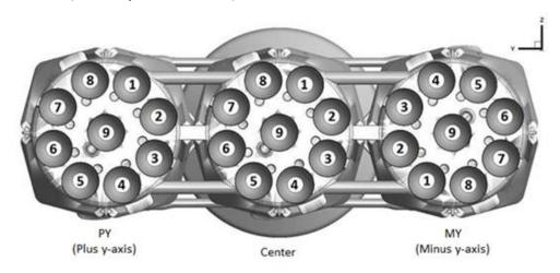
Figure 2-3: Falcon Heavy first-stage engine layout
