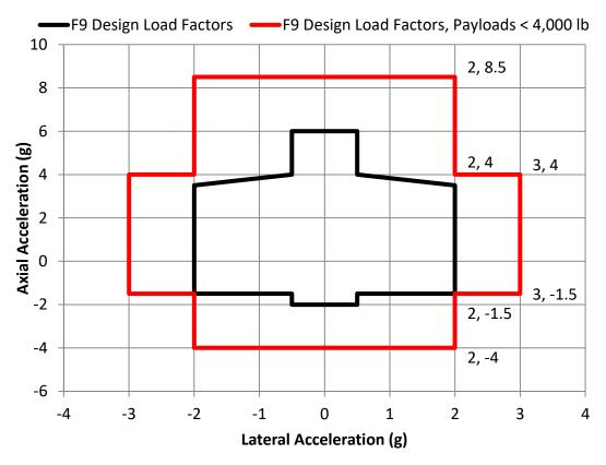
Figure 4-2: Falcon 9 flight limit load factors for light mass payloads (under 4,000 lb)
