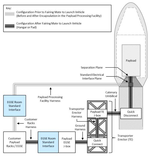
Figure 5-1: On-pad electrical interfaces
