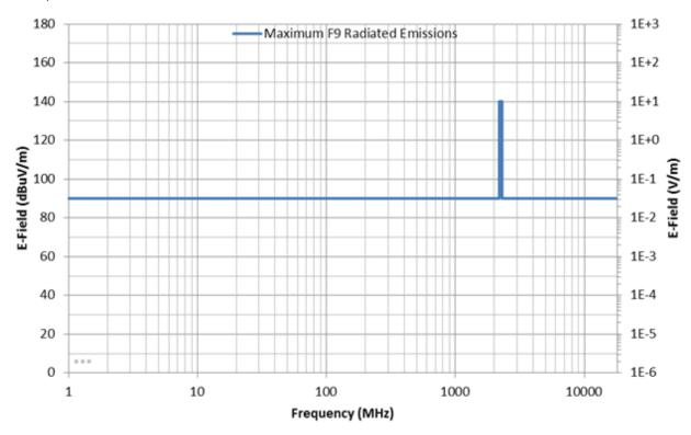
Figure 4-13: Falcon 9 worst-case radiated environment
