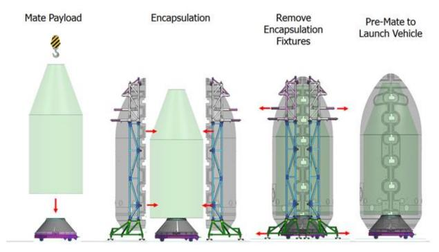
Figure 8-5: Payload encapsulation and integration sequence
