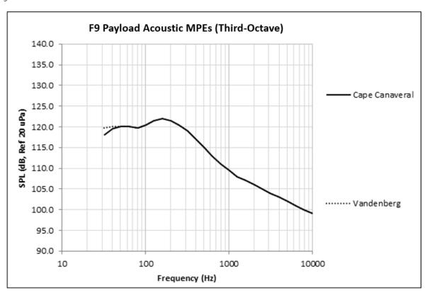
Figure 4-5: Falcon 9 maximum predicted acoustic environment (P95/50), 60% fill-factor, 131.3 dB OASPL (Cape Canaveral) and 131.4 dB OASPL (Vandenberg) in third octave, with fairing acoustic blankets
