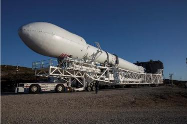
Figure 8-6: Integrated Falcon 9 on the transporter-erector within the integration hangar and rolling out
