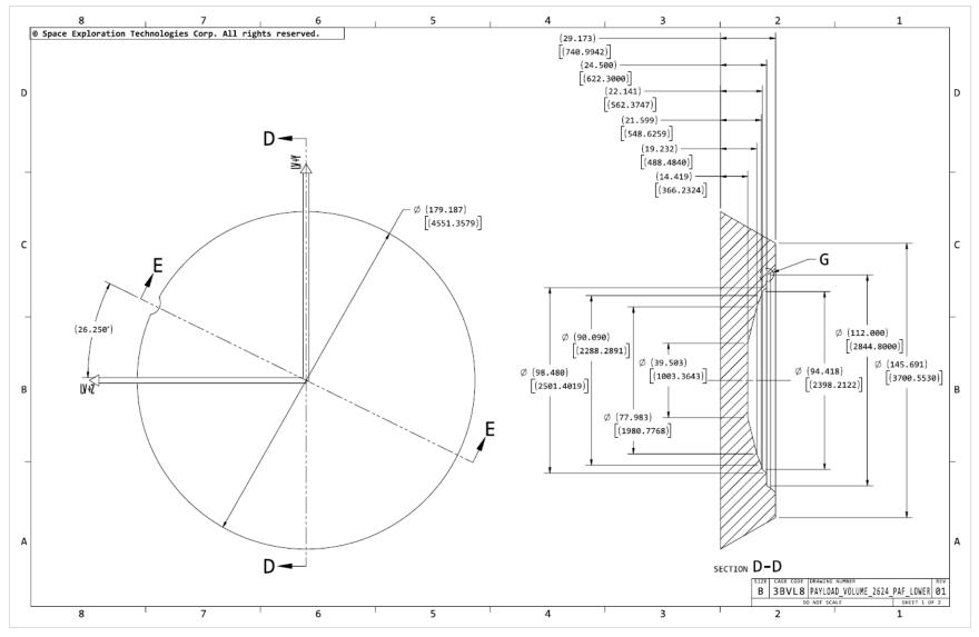
Figure 12-8: Payload lower volume, with 2,624-mm PAF (1 of 2)
