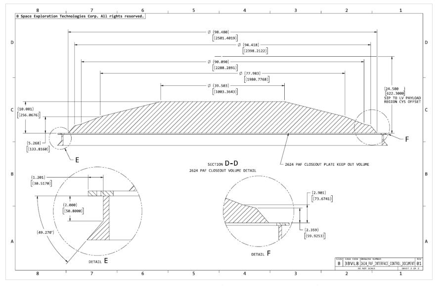
Figure 12-4: 2,624-mm interface drawing (close-out offset and keep-out volume)
