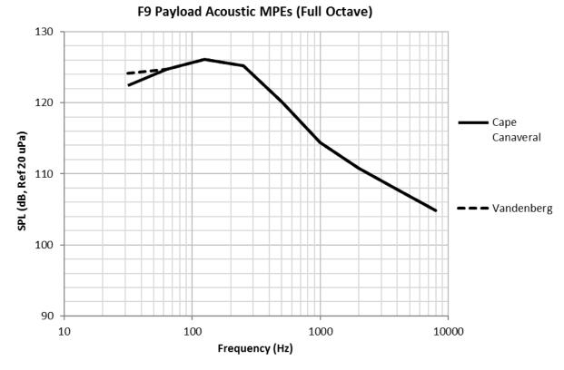
Figure 4-6: Falcon 9 maximum predicted acoustic environment (P95/50), 60% fill-factor, 131.4 dB 0ASPL (Cape Canaveral) and 131.6 0ASPL (Vandenberg) in full octave, with fairing acoustic blankets
