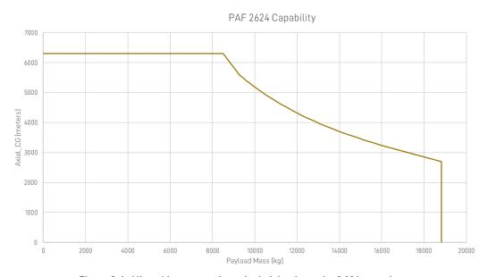
Figure 3-4: Allowable center-of-gravity height above the 2,624-mm plane
