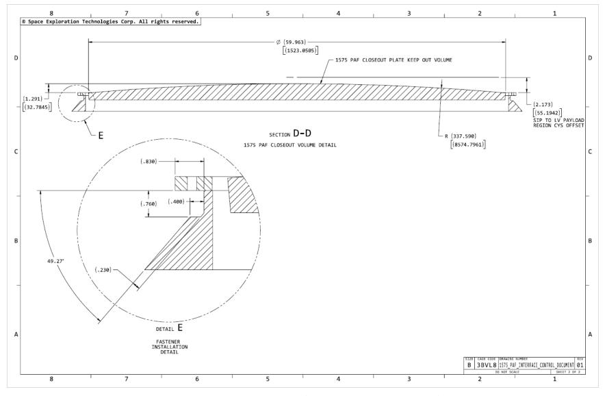
Figure 12-2: 1,575-mm interface drawing (close-out offset and keep-out volume)
