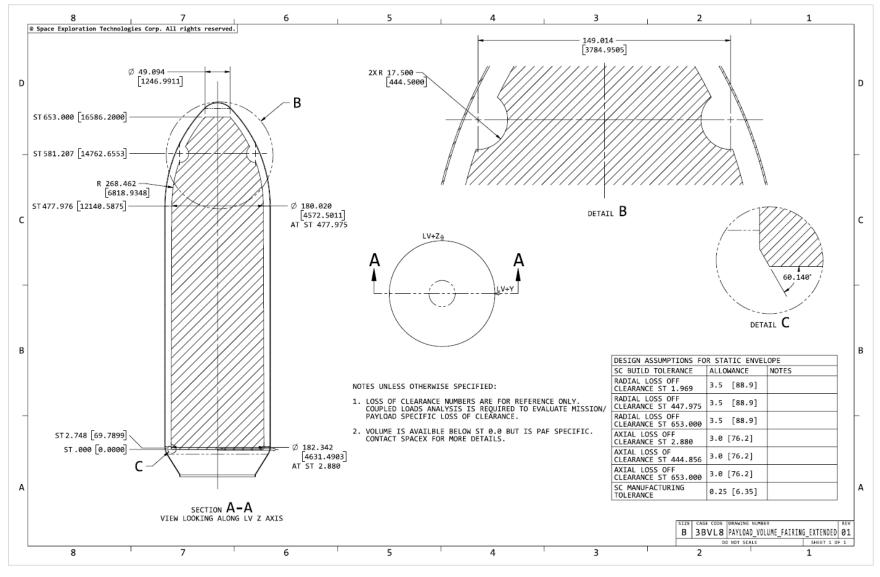
Figure 12-10: Falcon extended fairing with payload static envelope
