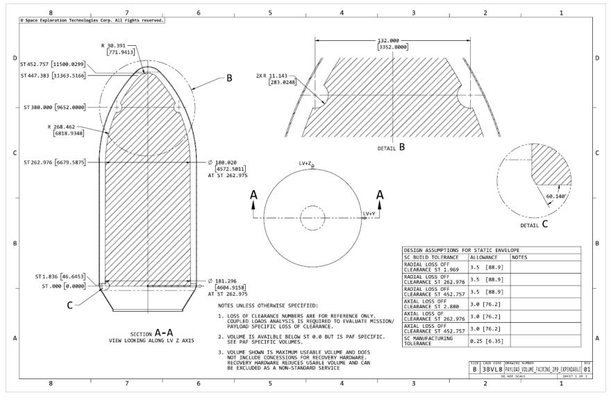
Figure 12-5: Payload static envelope (standard Falcon fairing)
