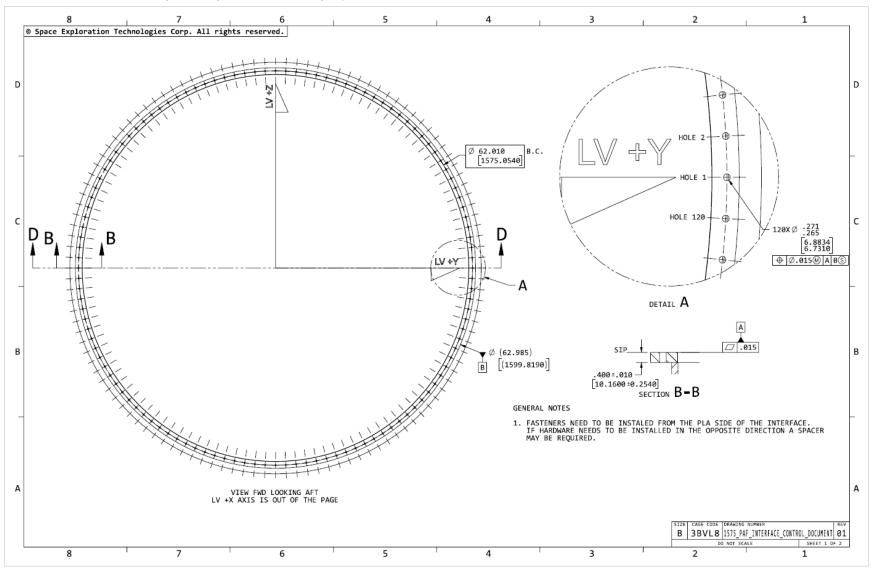
Figure 12-1: 1,575-mm interface drawing (interface plane details)
