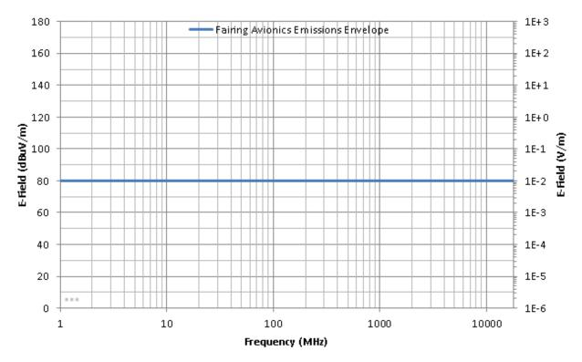
Figure 4-16: Fairing avionics emissions envelope
