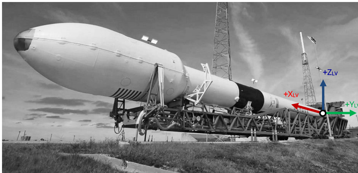
Figure 4-1: Launch Vehicle Coordinate Frame
