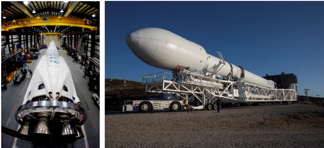
Figure 10-7: Falcon 9 on the Transporter-Erector in the Integration Hangar and During Rollout
