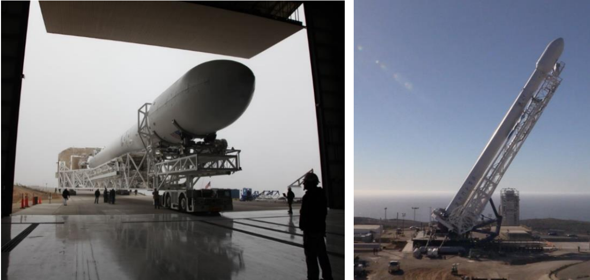
Figure 10-10: Launch Vehicle Rollout and Erection
